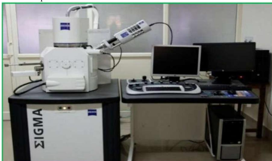
Figure:4 Photography diagram of field emission scanning electron microscope.
