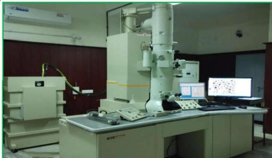
Figure:5 HR-TEM transmission electron microscope instrument.
