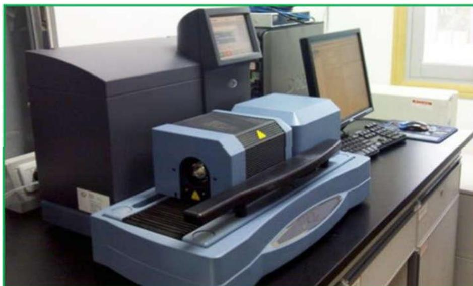
Figure:6 SDT Q600 Thermogravimetric Analyzer.
