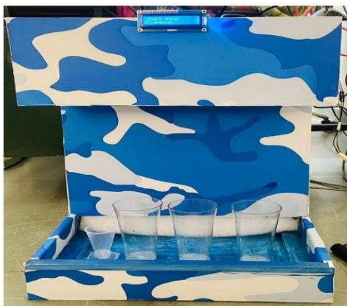
Fig 6.1: Proposed model of voice and gesture based Hot/Cold water dispenser Juice and Syrup dispenser system in health care using IOT
