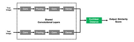
Figure 2: Architecture of a Siamese Neural Network
