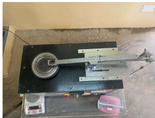
Fig.5 Wear Testing Machine
