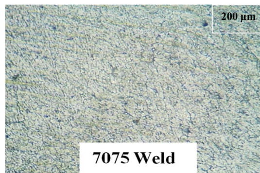
Figure 21. Microstructure of AA7075 metal, Figure 22. Microstructure of AA7075 metal and weld zone
