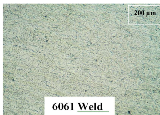
Figure 20. Microstructure of AA6061-AA6061 weld zone
