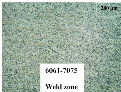
Figure 26. Microstructure of AA6061-AA7075 zone
