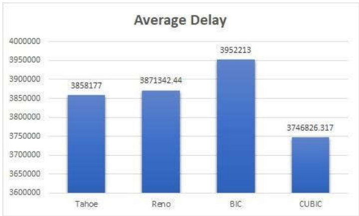
Fig. 9 Average Delay for different congestion control algorithms
