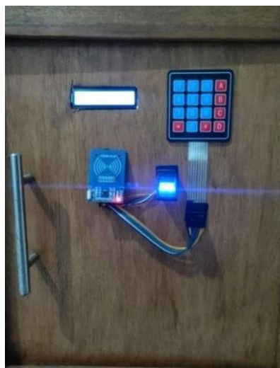
Figure 13. Complete device prototype of 3-level security system (front-view)
