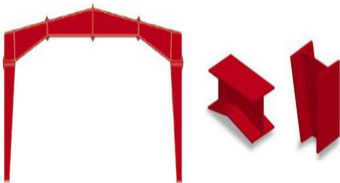
Figure 1. Built-Up “I” Shaped Primary Structural Framing Members.
