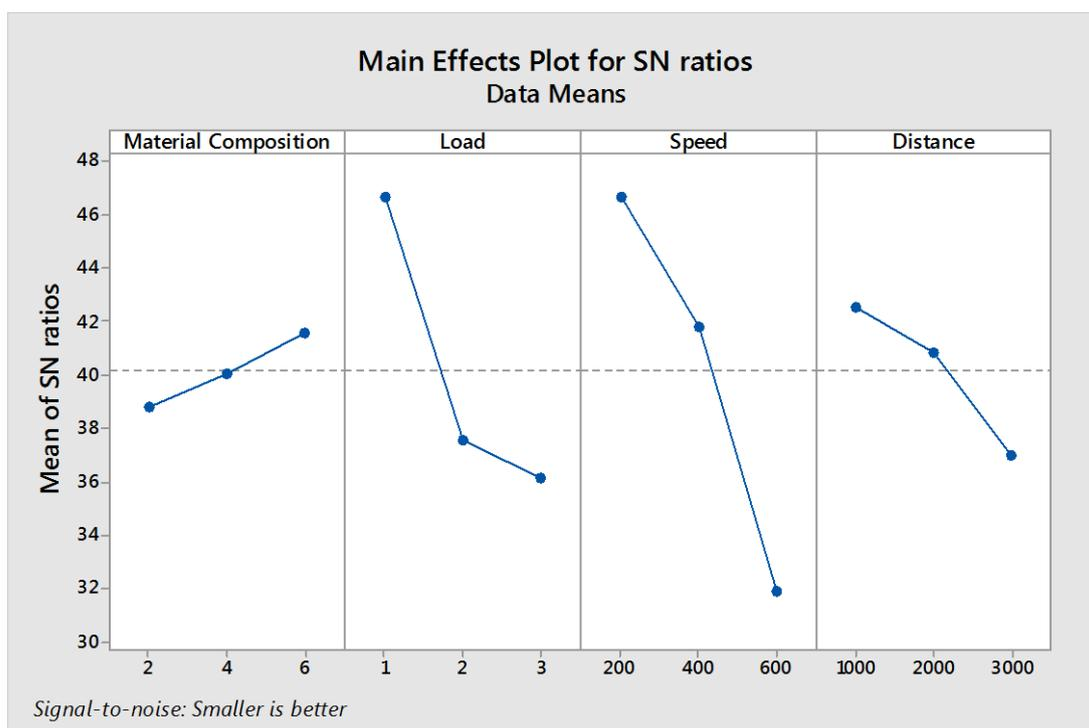
**Fig. 4: Main effects graph for SN ratios – Material loss**
