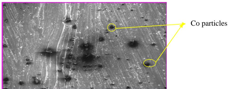
Fig. 3: Microstructure of Bronze - 6 wt.% Co
