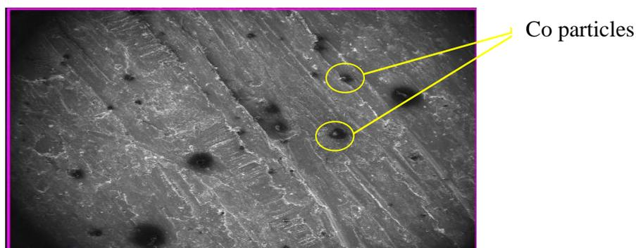
Fig. 2: Microstructure of Bronze - 4 wt.% Co
