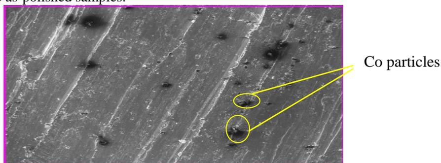
Fig. 1: Microstructure of Bronze - 2 wt.% Co
