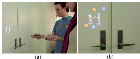
Figure 1. (a) Users hold micro projector-camera devices to project animated characters on the wall. (b) The characters recognize and interact with one another.
