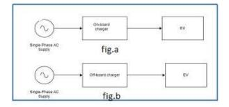
Fig. 1 a) On board charger b) Off-board charger
