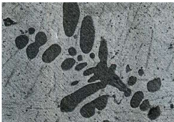
Figure 6 shows Microstructure of Sn-Zn-Al-La solder prepared by the author's research group.[6]
