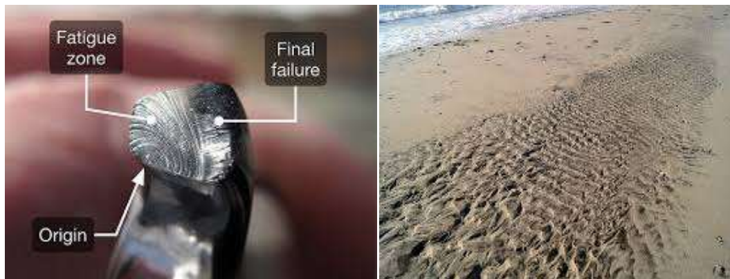
Figure 3 shows comparison between Beach marks in fatigue failure and Actual beach marks
