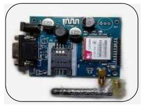
A GSM module is a special electronics circuitry which provide slot to insert SIM card and operates over a prepaid subscription, to the mobile operator, as a mobile phone. i.e. GSM Module can be used like a phone.
