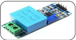
ZMPT101B AC Voltage Sensor, most suitable voltage sensor, provided where accurate measurement of AC voltage is highly required.
